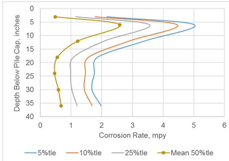
Figure 3 - Pile corrosion rates with depth below pile cap
