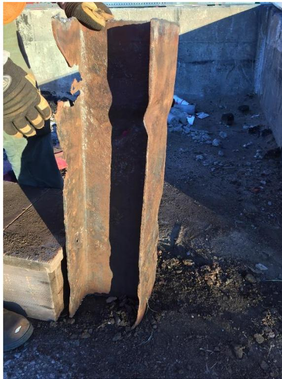
*Figure 2 – Pile fragment showing flange buckling caused by corrosion*
