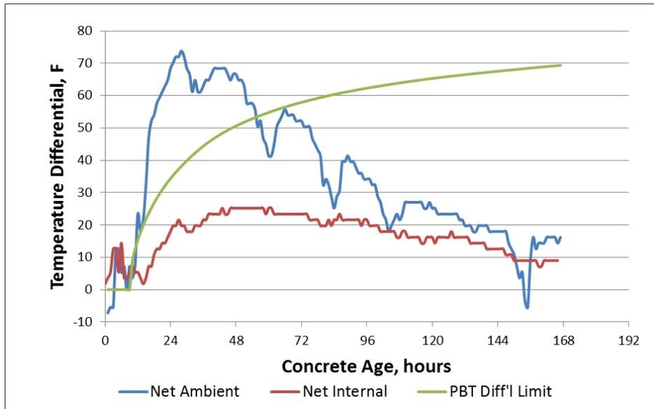
Figure 4 - Thermal monitoring of concrete during curing
